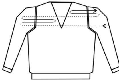
With a tank top or vest, the yarn carriers may not switch layers (front/back), so that no connections arise and remain open at the arm openings.
