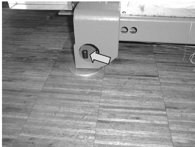
Fig. 4-12 Grub screws for aligning the machine
