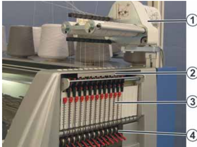
Fig. 2-8 Lateral yarn guide
