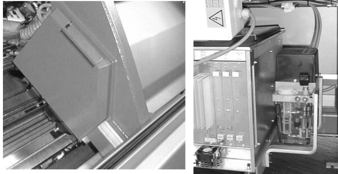
Fig. 2-16 Central lubrication on carriage, on the right: Oil supply
