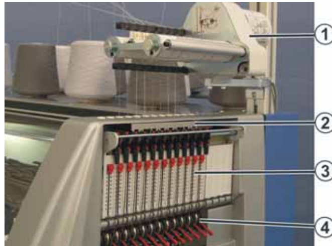
Fig. 2-6 Lateral yarn guide
