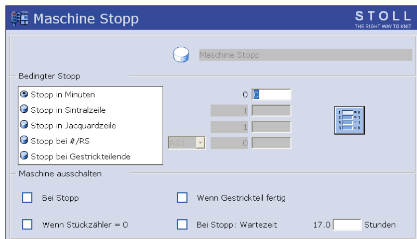
Fig. 3-22 Fenster "Maschine Stopp"
