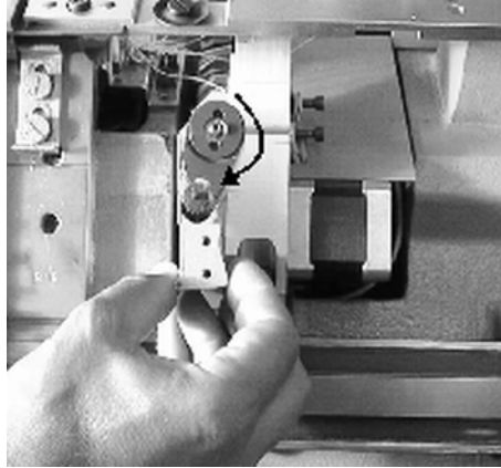
Fig. 5-26 Basic position of transport segment
