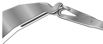
Fig. 4-60 Transfer position of transfer part and needle hook
