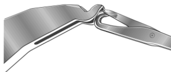
Fig. 4-58 Transfer position of transfer part and needle hook
