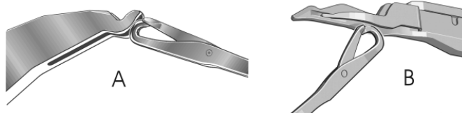
Fig. 4-51 Transfer position of transfer part and needle hook
