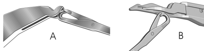
Fig. 4-53 Transfer position of transfer part and needle hook
