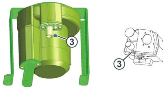
Fig. 4-5 Adapting fluff absorption (on the left: from component type 001 on, on the right: component type 000)
