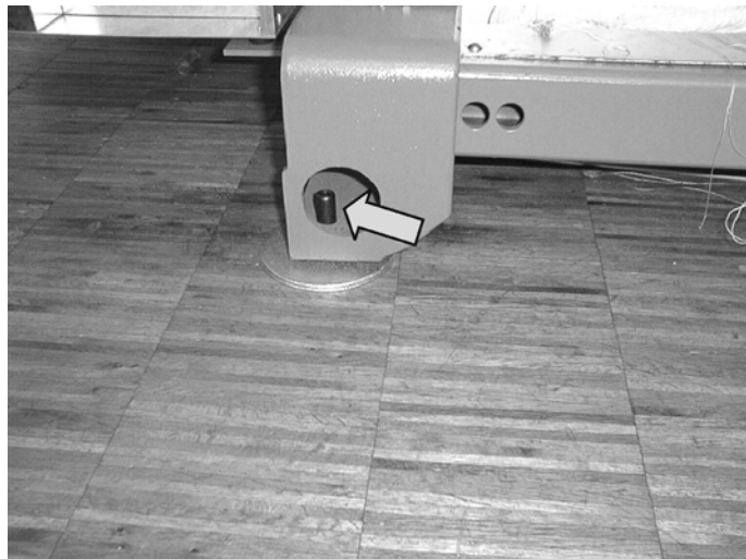
Fig. 4-12 Grub screws for aligning the machine
