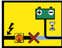
Fig. 4-42 "Power failure" pictograph
