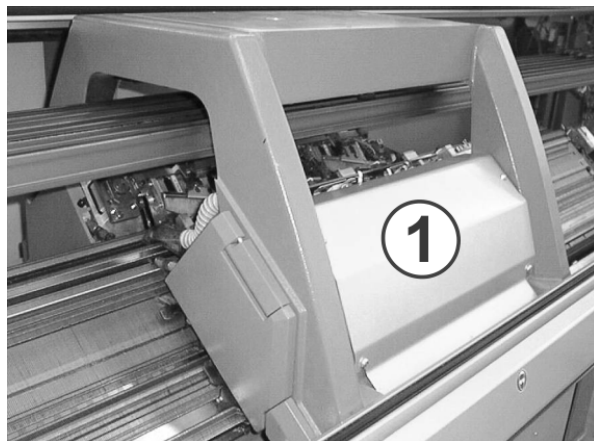
Fig. 6-29 Cover of carriage assembly
