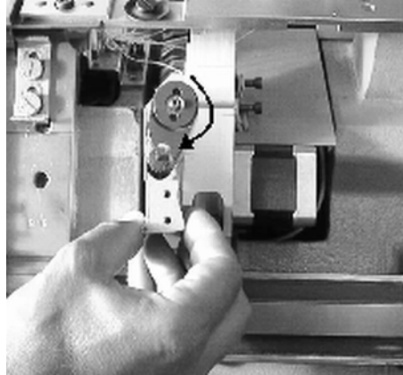
Fig. 5-19 Basic position of transport segment
