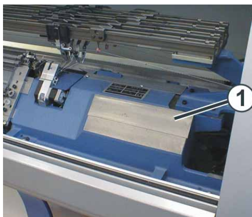
Fig. 6-34 Support surface of carriage part
