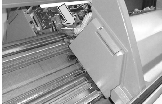
Fig. 2-14 Fluff absorption and lint container
