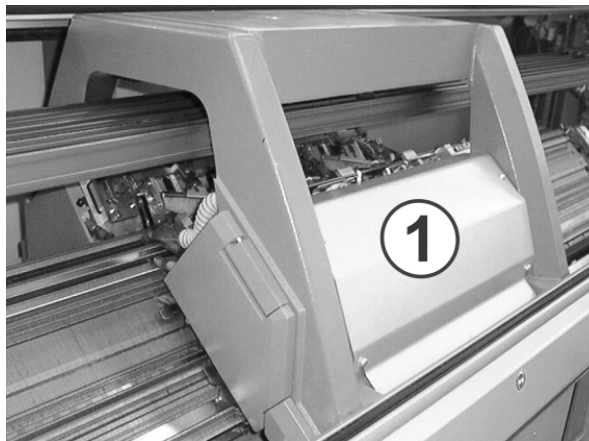
Fig. 6-25 Cover of carriage assembly
