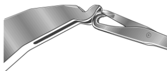
Transfer position of transfer part and needle hook
