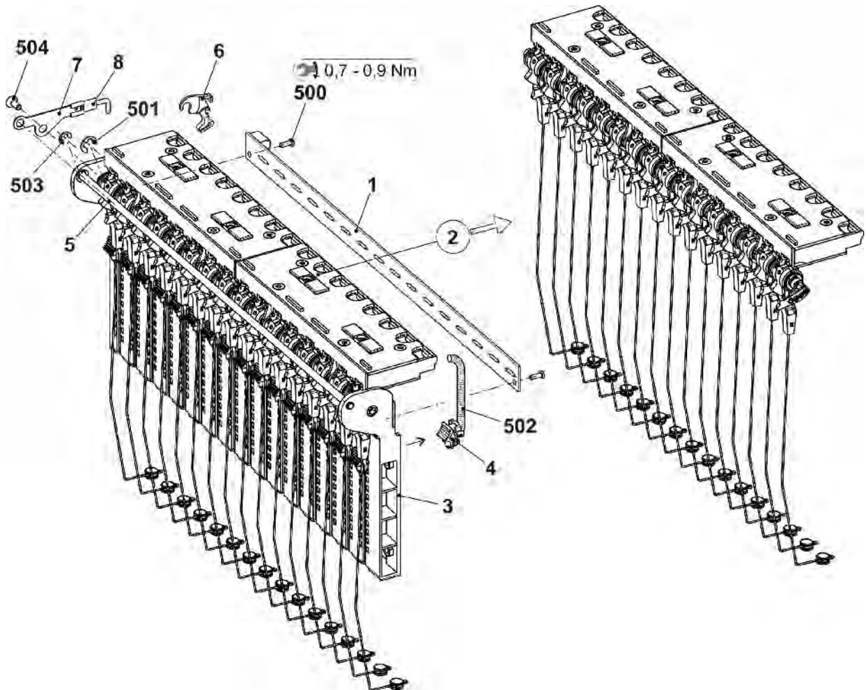
17.9.1.1 Tension axle E10 | E12 | E14 | E16 | E18 | E7.2 | E8.2 | E6.2(12m.10)
