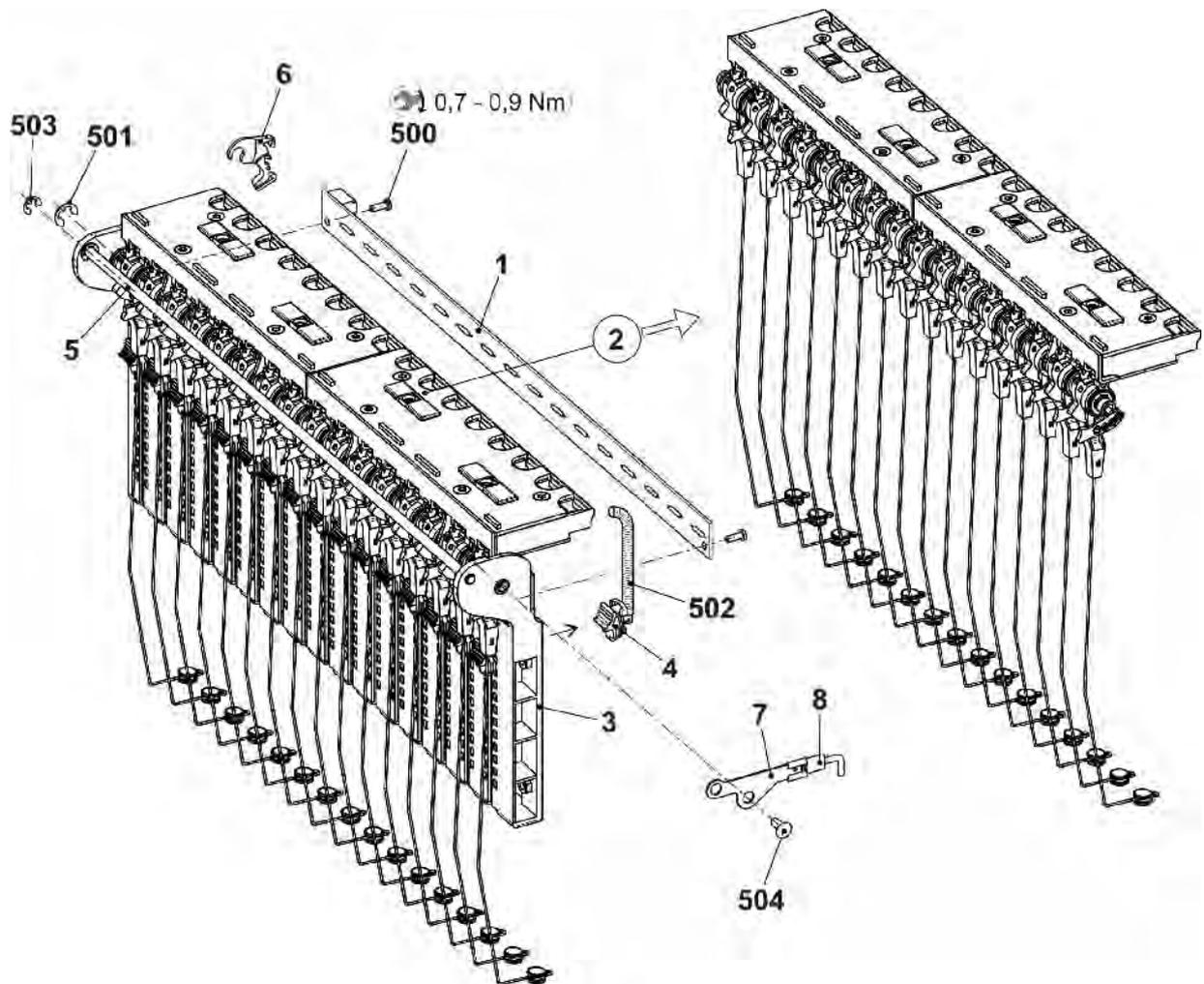
17.10.1.1 Tension axle E10 | E12 | E14 | E16 | E18 | E7.2 | E8.2 | E6.2(12m.10)
