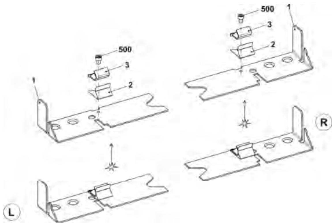
7.2 Yarn brake at clamping and cutting bed
