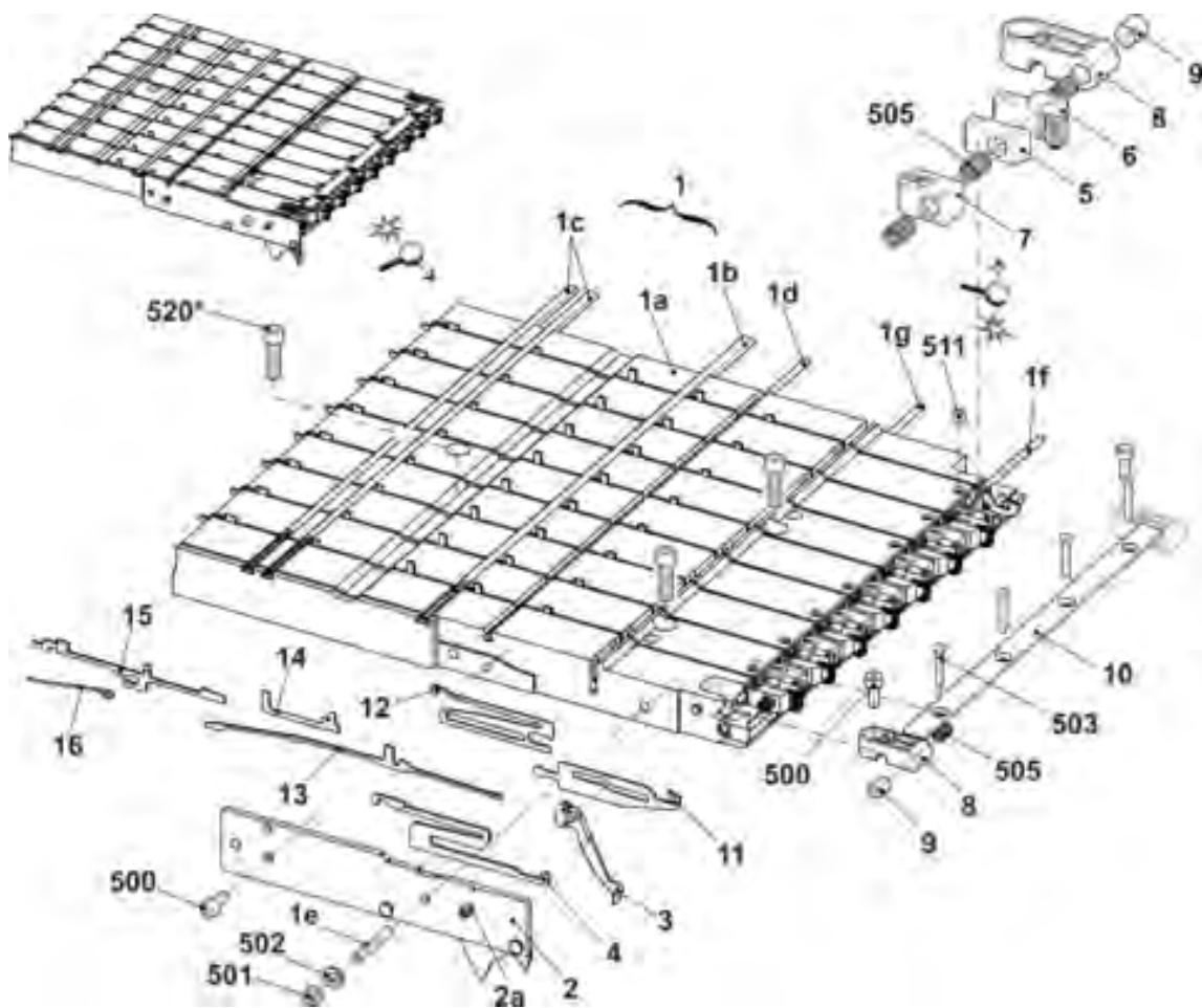
4.18 Right clamping and cutting bed E5-7 | E5m.4 | E7m.5 | 7m.8 | E2,5.2 | E3,5.2 | E2,5.2 | E3,5.2 | E2,5.2m4L | E3,5.2m4L
