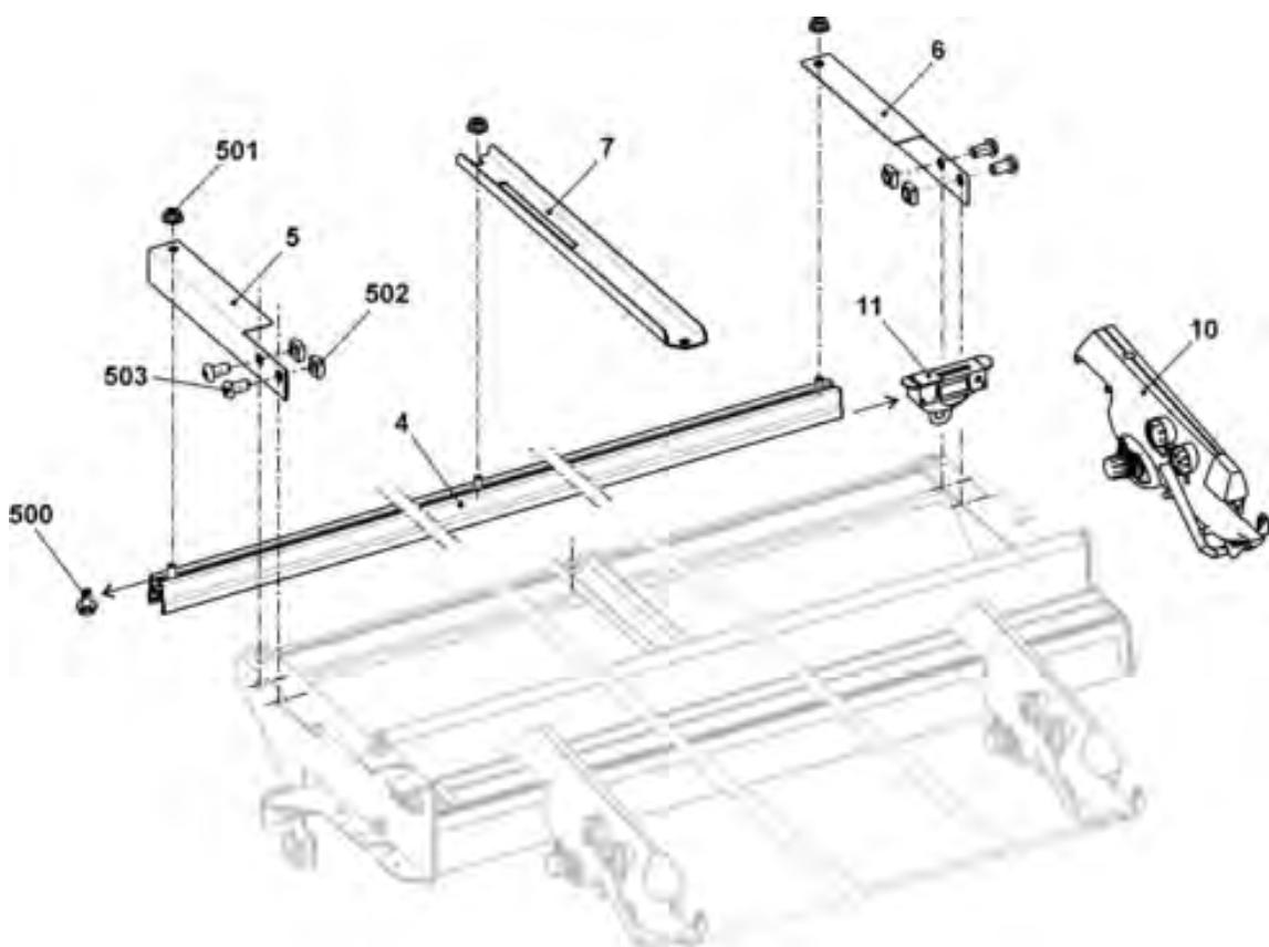
17.8 Friction feed wheel on the left and on the right complete
