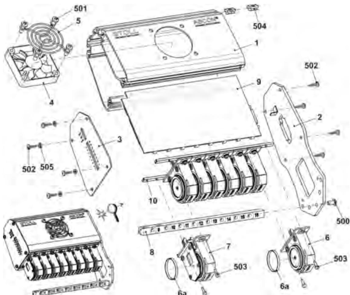
16.10 Yarn length measuring device on the right complete
