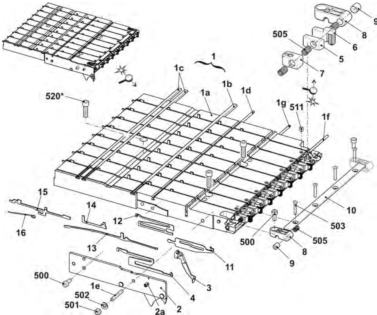
4.18 Right clamping and cutting bed E5-7 | E5m.4 | E7m.5 | 7m.
