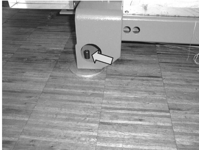
Grub screws for aligning the machine
