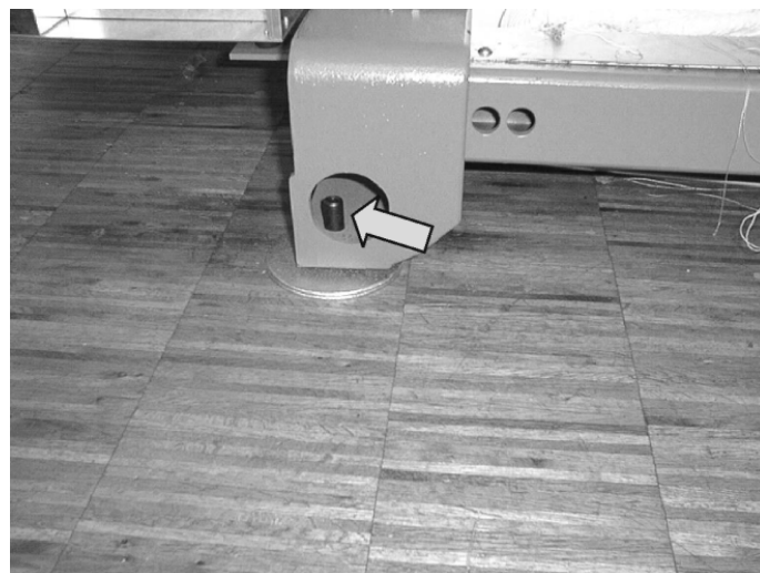
Grub screws for aligning the machine
