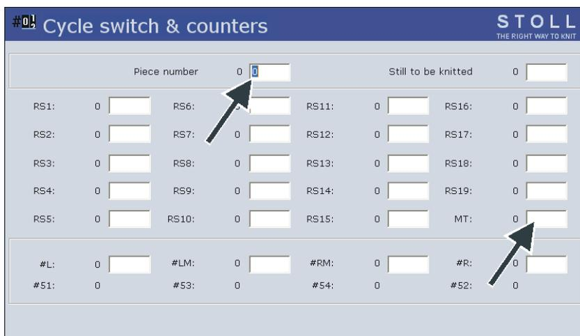
The screenshot shows the "Cycle switch & counters" interface. At the top, there are two main input fields: "Piece number" (set to 0) and "Still to be knitted" (set to 0). Below these are two columns of smaller input fields for individual row counters, labeled RS1 through RS19, and an "MT" field. At the bottom, there are four more input fields labeled #L, #LM, #RM, #R, #51, #53, #54, and #52. Arrows in the image point to the "Piece number" field and the "MT" field.
