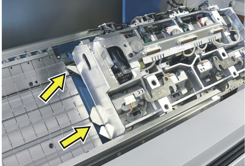
4. Push the carriage part inward and assemble with the carriage assembly.
