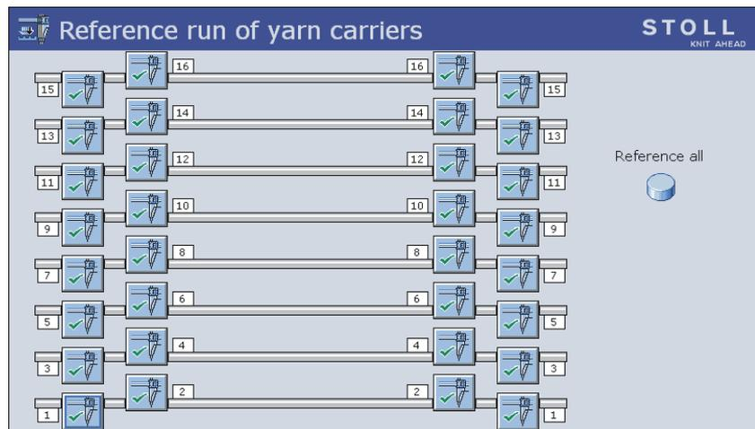
6. The reference run is complete, the machine is ready to knit.
