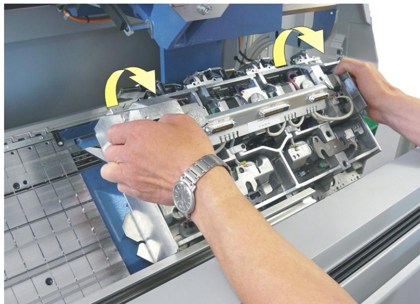
3. If the outer cams are positioned above the clamping and cutting bed, position the carriage part on the support surface.
