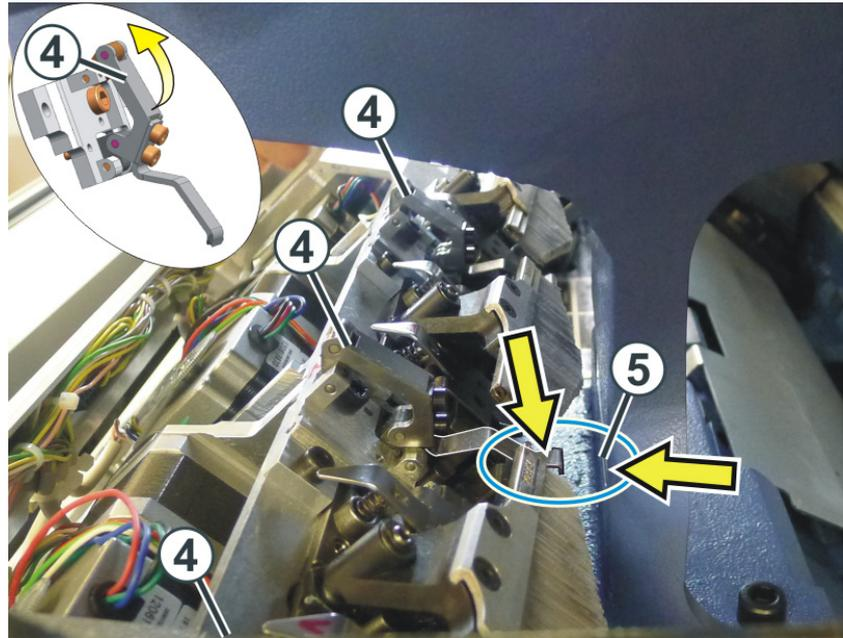
2. Push the carriage part from outside on to the support surface (1). To prevent the presser feet from colliding with the support (5) lift the carriage part somewhat and push it inward.
