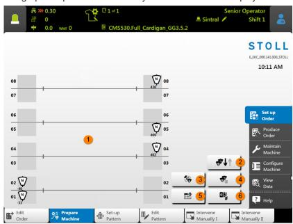
**1** Graphic display of the active yarn carriers of the yarn carrier home position of the loaded knitting program.
