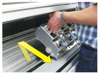
With the front carriage part there is the risk of the cover being damaged if the carriage part is lifted off directly from the needle bed.
