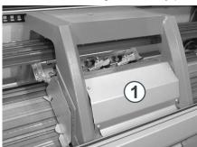
4. If the rear carriage part is removed, the needle detector is to be removed as well.
