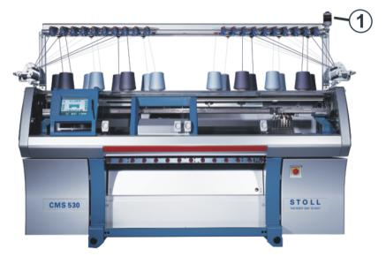
The signal light (1) displays the operating status (green, yellow) of the knitting machine.
