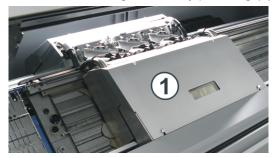
4. Push the locking of the fluff container downwards and pull away container upwards.
