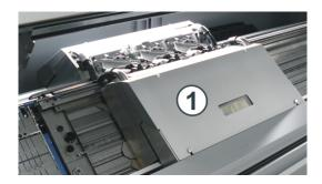
2. Grease the lubricating nipples (2) with a grease gun (Stoll Grease 475)
