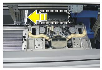
5. Remove the carriage assembly panelling (1).
