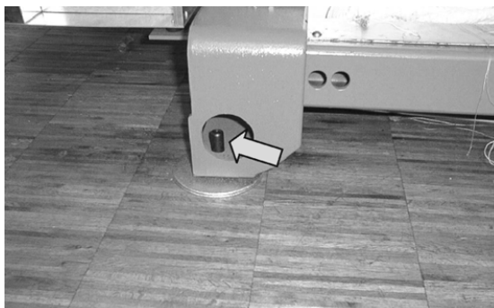
Setscrews for aligning the machine
