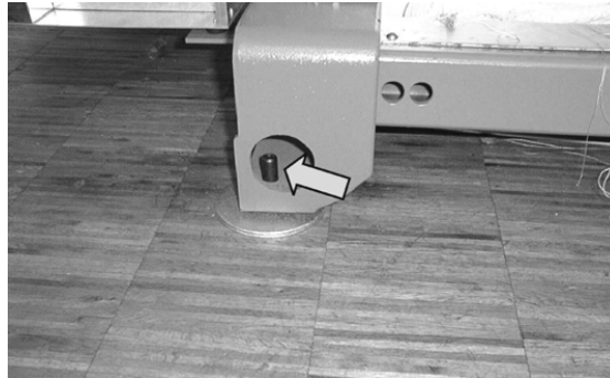
Setscrews for aligning the machine
