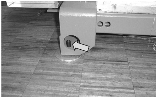
Setscrews for aligning the machine
