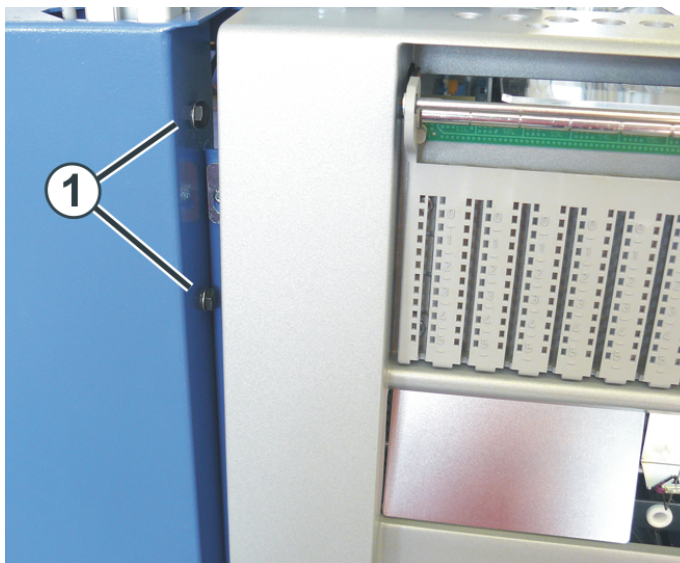
Supports for the yarn guide device
