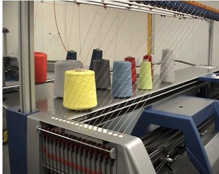
5. Lead all threads for a yarn carrier on this side via the same track of the yarn deflector.
