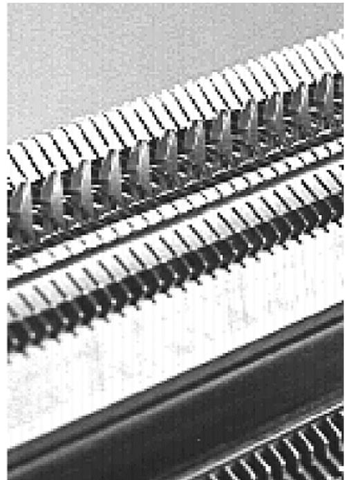
**Comb hooks with the sliders open or closed:**
