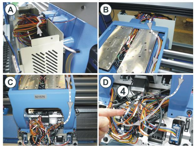
11. Plug the cable into the socket (4) of the front needle detector (image D).
