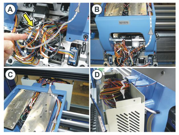
8. Plug the new cable (ID 4170 283 054) into the "CN8" socket (3).
