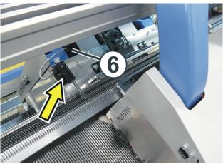
12. Screw the needle detector tight on the rear carriage.
