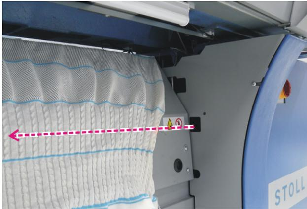
The light barrier is switched on with the "LW1" command and switched off with "LW0".
