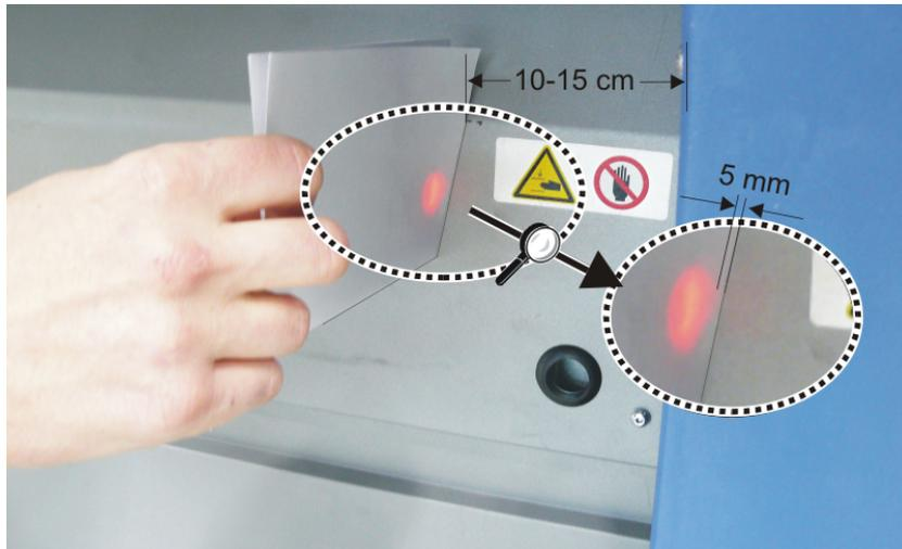
16. The setting is correct when the outer edge of the light beam is around 5 mm from the edge of the paper.
