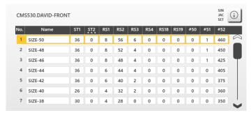
A knitting order (line) is processed until the number of fabrics in the "ST1" and "ST2" columns are the same. The machine automatically switches over to the next size and produces the set piece number. Knitting is carried out line by line from top to bottom.
