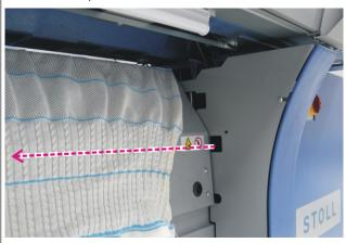
The light barrier is switched on with the "LW1" command and switched off with "LW0".
